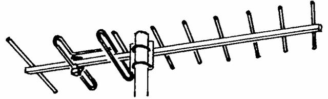
The Yagi dipoles and parasitic elements are match marked to the supporting crossarm. The antenna main mounting clamp holes are located in the crossarm perpendicular to the element holes. The dipole insulators and parasitic elements mount to the same side of the crossarm.
