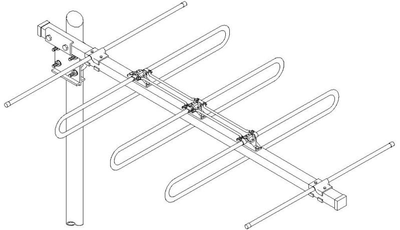
The Yagi dipoles and parasitic elements are match marked to the supporting crossarm. The antenna main mounting clamp holes are located in the crossarm perpendicular to the element holes. The dipole insulators and parasitic elements mount to the same side of the crossarm.
